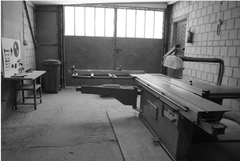
Fig. 3. The cross- cut and mesh circular saw station after the implementation of 6S. [3]
